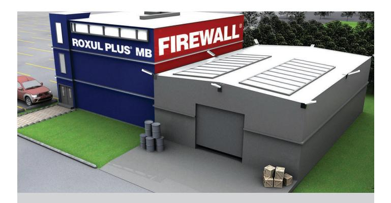
ROXUL FIREWALL® and ROXUL PLUS® MB products are used to insulate walls in pre-engineered metal buildings. ROXUL FIREWALL is ideally suited for zero lot line applications where buildings are in close proximity and fire safety is essential.
